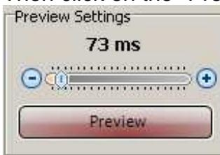
The exposure duration can be set with the cursor. The unit is ms (milliseconds).
