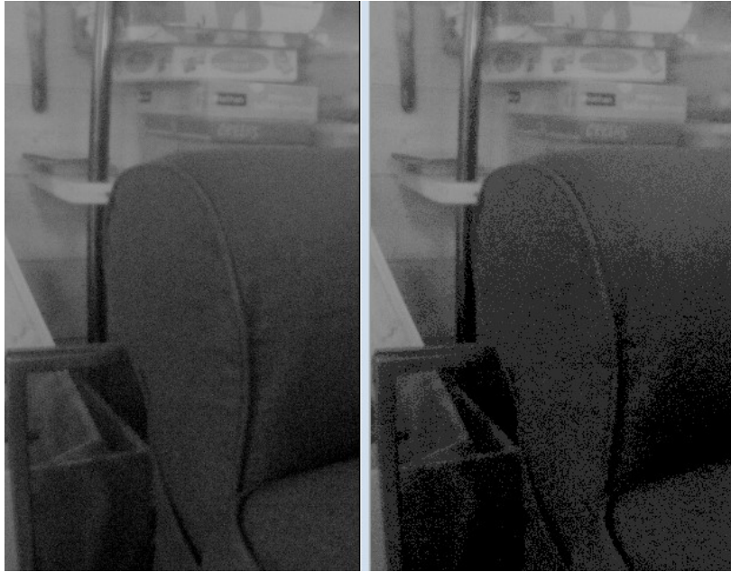
Figure 1 – playing at daytime with the 12-bit (left) and 8-bit (right) modes. The posterization effect is dramatically diminished in 12 bits. This has no effect on planetary and lunar imaging (at the exception of delicate features such as dark, lunar domes near the terminator), but the 12-bit mode is a serious advantage to image deep-sky objects such as diffuse nebulae or galaxies which show limited contrast.
