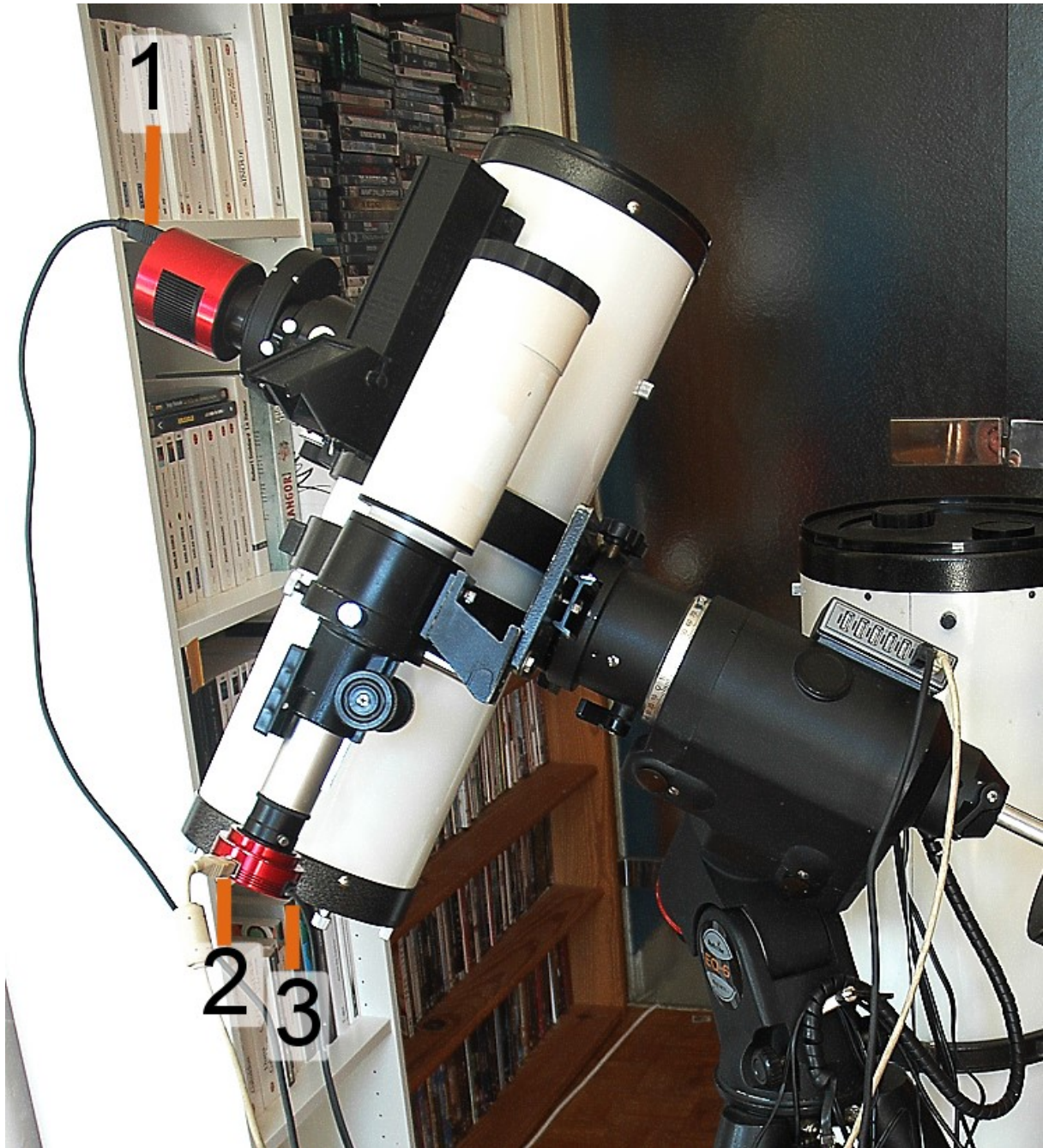
Figure 16 – The ASI120MM as an autoguider. (1) a cooled ASI with its USB cable (the power supply cable for cooling is not represented). The ASI120MM has two connectors : (2) the USB2 cable to the laptop with autoguiding software such as PHD2, and (3) a RJ11 cable for the corresponding connector on the mount, labelled « autoguider ». This is only one possibility amid many others. It is better to rotate the ASI120MM so that the image is aligned horizontally with the right ascension. When the motors of the mount are off, the guide stars have to drift horizontally. Then the motors are set on, the software completes an automatic calibration, and the autoguiding is operational. Despite its small sensor, the ASI120MM is sensitive enough to detect guide stars even if the guide scope cannot be orientated independently from the imaging telescope. The ASI120MM runs with PHD2 with the ASCOMV2 driver, RAW8 mode. Image N. Dupont-Bloch.
